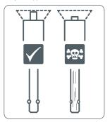
Figure shows left pin in good working condition. The right pin should be retired due to wear and detent pins not properly working.
